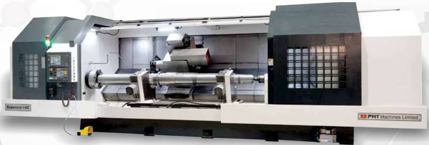
CNC Turning Center 5000 ABC with C/Y axis & live tools
