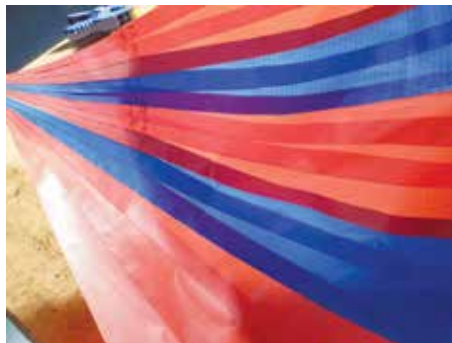
Spinnaker assembled before seaming
