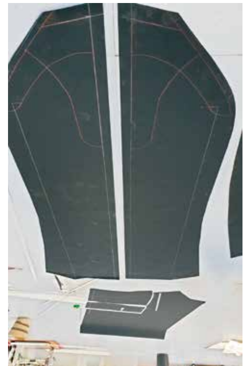
After careful measurements on board, a boom bag is lofted by hand.
