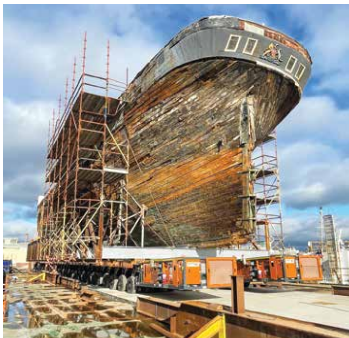
Two lines of SPMTs lifting cradle and ship ready for Offload
