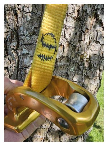
As with all life critical and aerial access kit, a good inspection regime should be observed, with pre and post used inspections in addition to mandatory, regulatory inspection and record keeping as required. Key inspection points should include the straps and associated stitching, the strap retaining screw is secured correctly and the pulley sheave operates smoothly. Also check the metal parts: absence of deformation, cracks, marks, wear, dirt, abrasion and corrosion.
