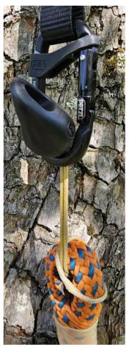
this you are readying the system for remote retrieval, from the ground. At this stage vou may also choose to attach a throwline to the provided loop on the back of the black retrieval sling. You may elect to re-ascend to your TIP on completion of aerial working, if you don't want the pre rigged throw line during working operations getting in the way. Petzl recommend the use of a soft retrieval, thus preventing the NAJA from falling to the ground, and possibly being damaged.
