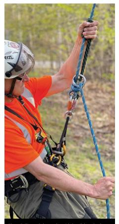
Photo 3: Figure-8 descender with Prusik loop backup.
