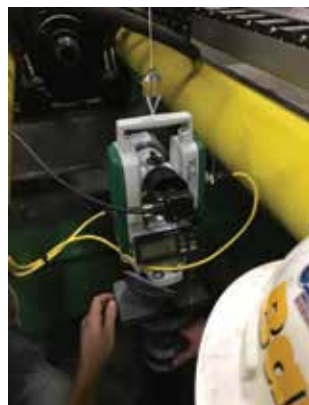
Figure 7.3.1.4 - Theodolite is matched to the plum bob.
