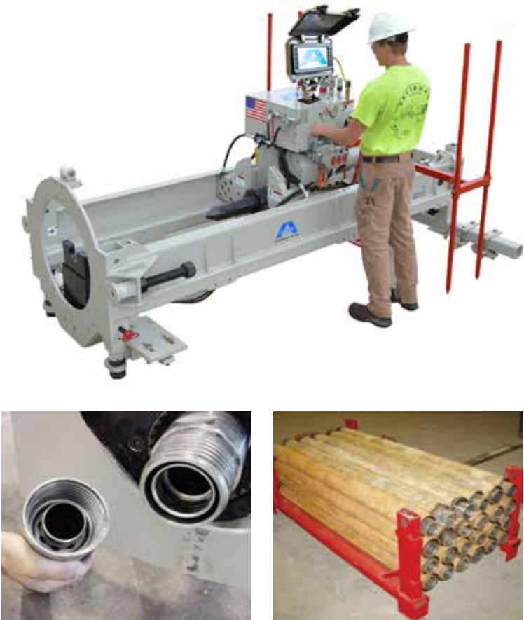
Figure 7.3.2.2.1 - Pilot tubes with threaded and hex connections.
