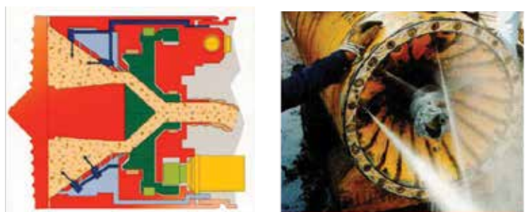
Figure 6.13 High pressure flushing system in the crushing chamber.
