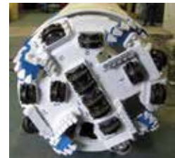
Mixed Ground Cutterhead, 6.5" Discs, SBU
