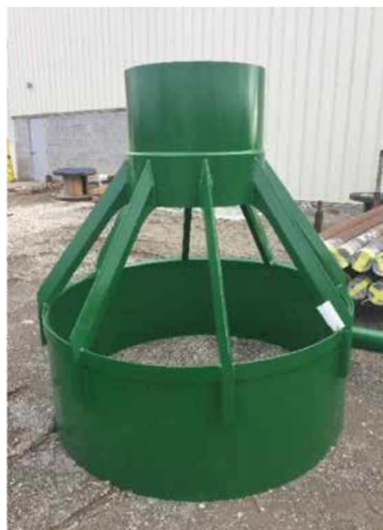
Figure 7.3.4.2.1 - Soft soil step reaming head known as a Transition Reamer.
