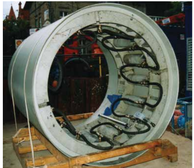
Figure 6.17 Intermediate sealed jacking station.
