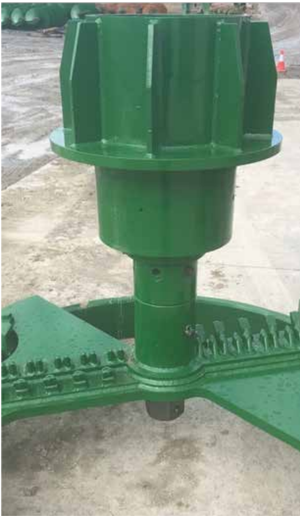
Figure 7.3.4.2.3 - Casing Thrust Swivel connected to conventional cutter head with pilot receiver.
