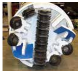
Rock Cutterhead 9.5" Discs, SBU
