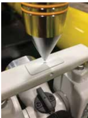
Figure 7.3.1.4 - Theodolite is matched to the plum bob.
