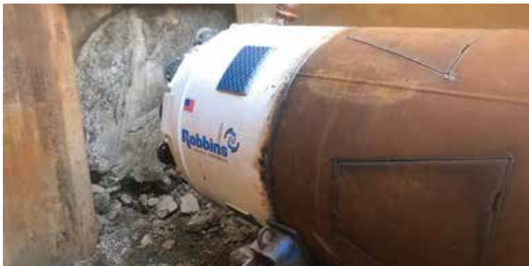
Figure 4.7 Steering shoes cut into lead casing. (Courtesy of The Robbins Company)
