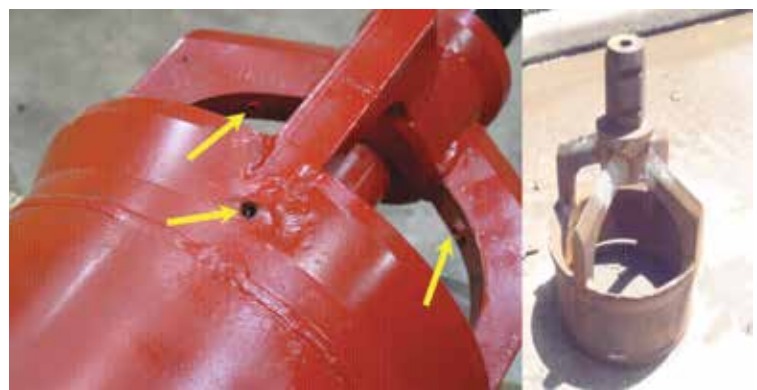
Figure 7.3.3.1.2 - Reaming Head or Cutting Head (also known as a Knife Reamer). Indicators point out lubrication ports.
