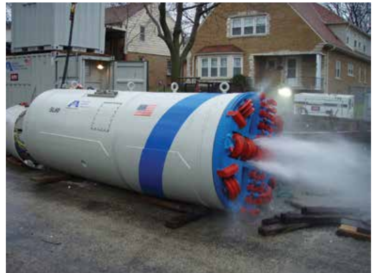
Figure 6.10 Akkerman SL60C with High-Pressure Jetting Nozzles.
