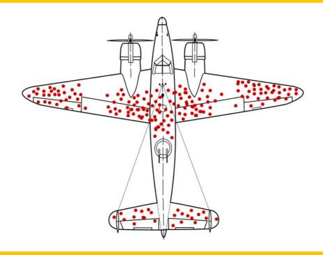
During World War II a few warplanes had returned after missions. It was decided to strengthen the planes by adding armour on them. After measuring the bullet holes on the warplanes it was found that the fuselage had the highest bullets per unit area followed by the wings and finally the tail. While common sense seems to dictate that we reinforce the fuselage the most, the statistician Abraham Wald steps in to save the day. He suggested that the areas with least damage be reinforced.
