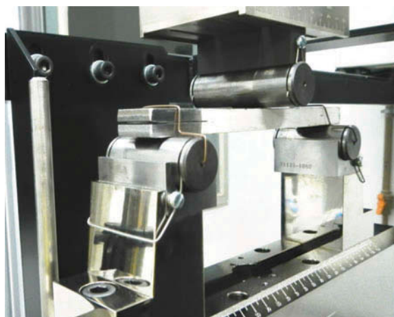
Figure 1. Illustration of specimen installation in servo-hydraulic machine.
