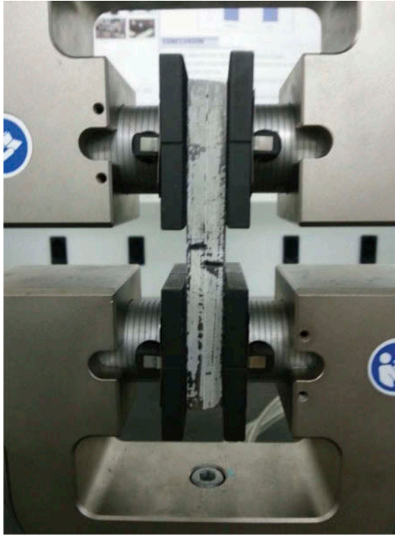
Figure 3. Thick adherend shear test setup in the testing machine.
