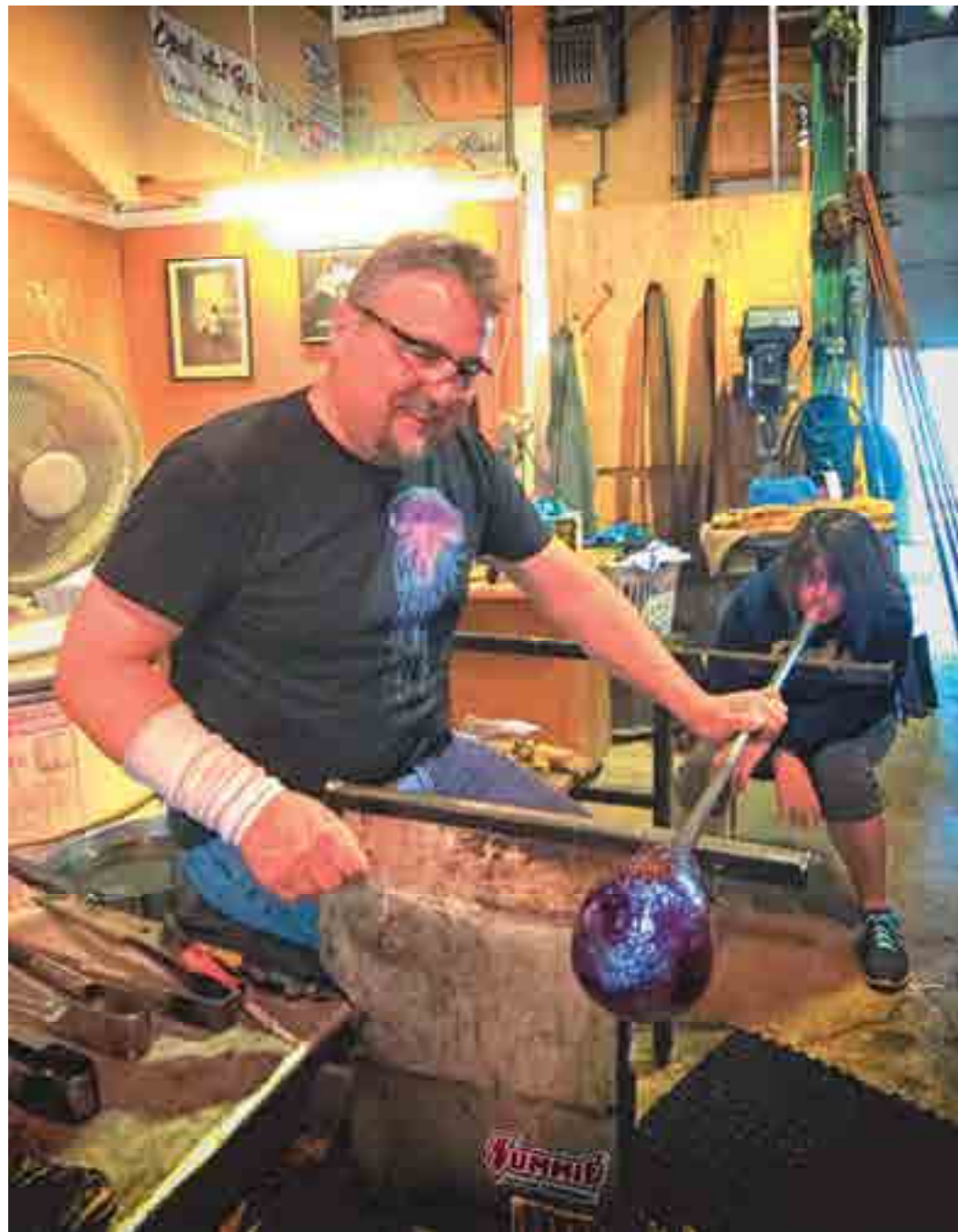
▶ Johnny dips the glass into crushed colored glass to add color.
