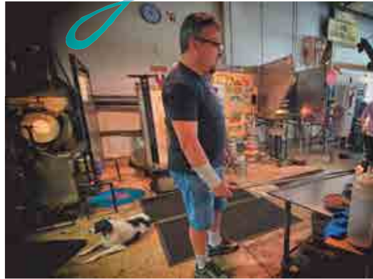
▶ Johnny is gathering molten glass in the furnace on the blowpipe. The furnace must be at least 2000° and is never turned off.
