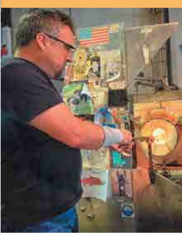
▶ Johnny is gathering molten glass in the furnace on the blowpipe. The furnace must be at least 2000° and is never turned off.
