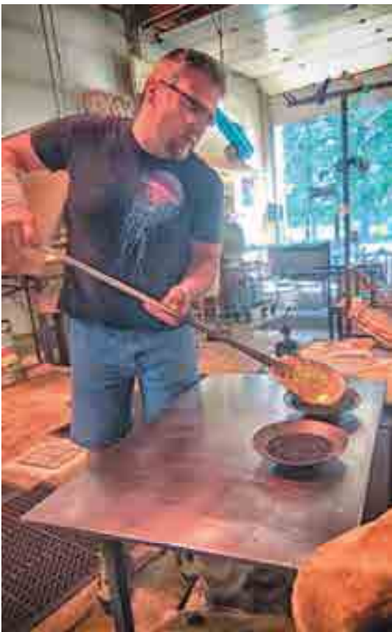
▶ Johnny dips the glass into crushed colored glass to add color.
