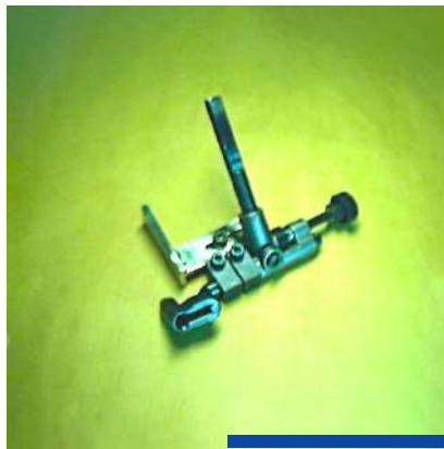
FCS 00011 Special guide for piping
