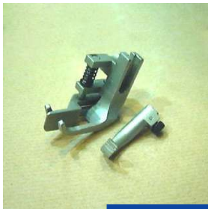
FCS 00014 Presser foot set for open stitch (PLC1610)
