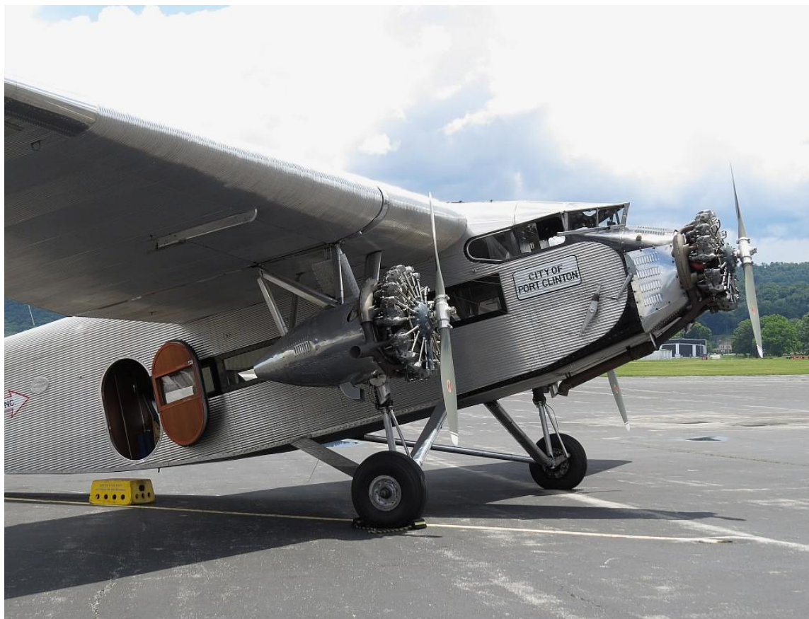
A close-up of the nose of the Liberty Aviation Museum's 1928 Ford 5-AT-B Tri-Motor during its recent visit to the Capital City Airport in Harrisburg, Pennsylvania. Some of the Ford Tri-Motor's unique features showcased in this picture include the three Pratt & Whitney radial engines, the wide-track main landing gear, the passenger cabin door, and the metal cables that actuate the control surfaces, visible just below the cockpit windows.
