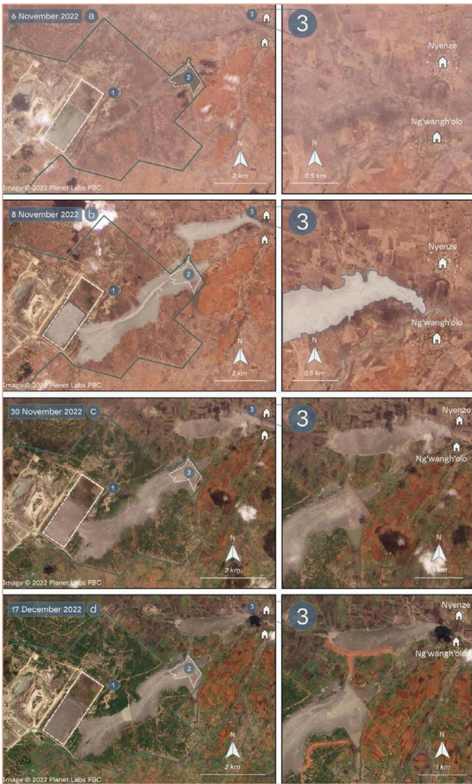
Planet satellite images of the 7 November 2022 tailings dam breach at the Williamson mine. The situation on the day before (a) and the day after (b) the dam breach.
