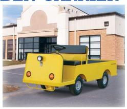
Taylor-Dunn's Loadmaster is durable, reliable and cost effective for your commercial and industrial material handling needs. Equipped with a 36-volt electric drive train, this vehicle carries loads up to 1,600 pounds at speeds up to 12 miles per hour with a range up to 20 miles.
