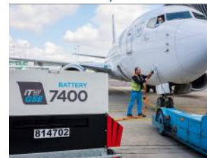
Electrical power of aircrafts at gates (Source: Schipol)
