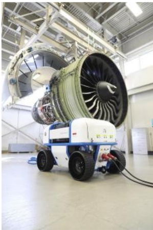
360 Engine foam wash, reduces emissions and improves exiting efficiency (Source: General Electric)
