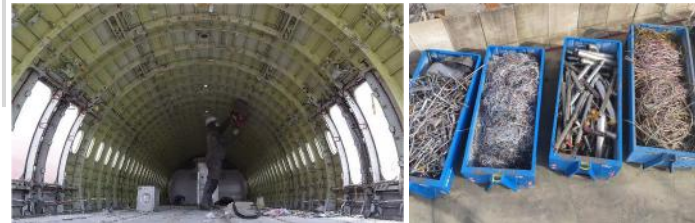
Aircraft end of life disassembly, material and components recovery and recycling (Source: Airbus)
