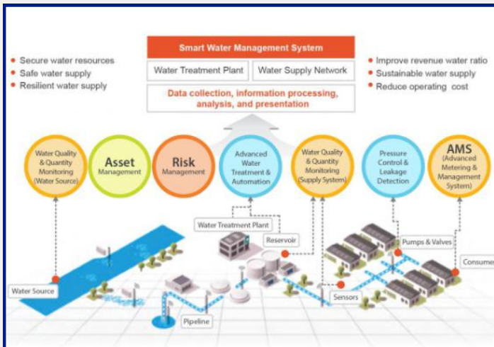
SMART WATER MANAGEMENT SYSTEM IN BIM
