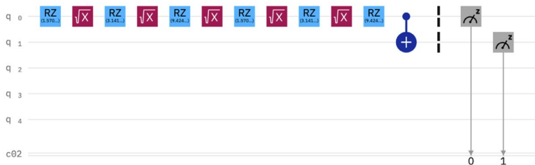
Left Figure 4: Circuit diagram of a Bell State with 0 identity gates conducted after being transpiled onto the 'ibmq_manila' system.
