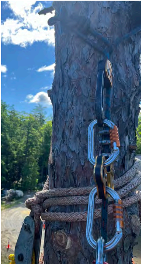
Photo 4: Backup climbing line, above, and rigging installed in adjacent red pine. Note running bowline and Yosemite tie-off on the climbing line.
