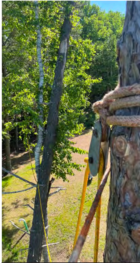
Photo 5: Rigging set with five-eighths-inch Hobbs Block (WLL 4,000pounds), three-quarter-inch Samson Tenex dead-eye sling (WLL 2,200 pounds) and five-eighths-inch Sterling Atlas rigging line (SWL 1,800 pounds, using a 10:1 safety factor).
