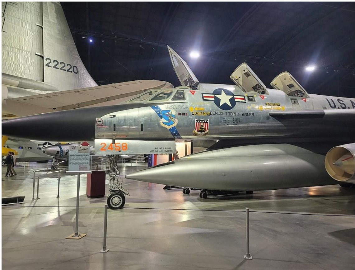
To keep the B-58 Hustler's profile as sleek as possible, the cockpits for the three crewmembers were separate and arranged in a tandem layout. The pilot sat in the front cockpit, the navigator/bombardier in the second cockpit, and the defensive systems operator in the rear cockpit. This photo also shows the two-component pod (TCP) mounted to the underside of the aircraft, which held most of the B-58's fuel and ordnance. (Image courtesy of Fast Eddie Leuter)
