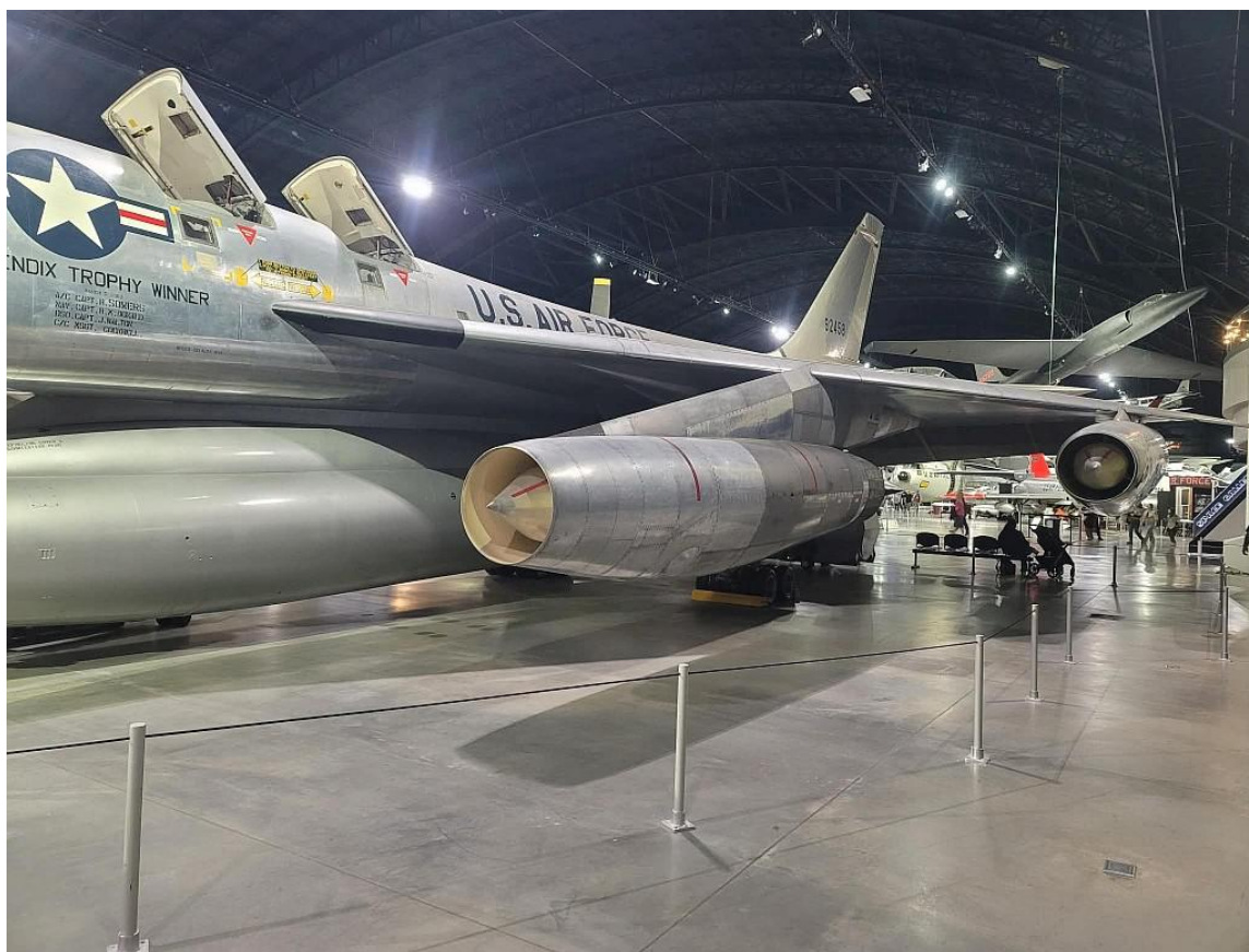
The B-58 Hustler was powered by four General Electric J79 axial-flow turbojet engines equipped with afterburners. These engines were optimized for supersonic flight and could propel the B58 Hustler to speeds above Mach 2, or twice the speed of sound. (Image courtesy of Fast Eddie Leuter)
