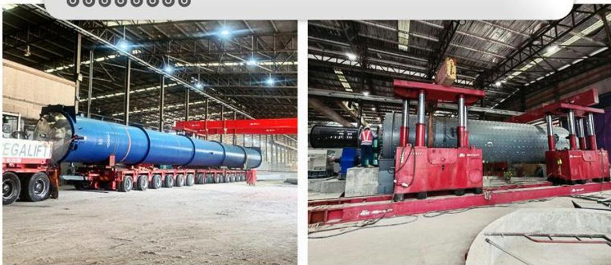
Megalift recently completed the safe and precise transportation of 4 massive Autoclave, each 33 meters long, from Port Klang to Perak. Using Megalift's 12-axle heavy transport system, the team ensured smooth delivery and executed offloading into the plant area using a gantry.
