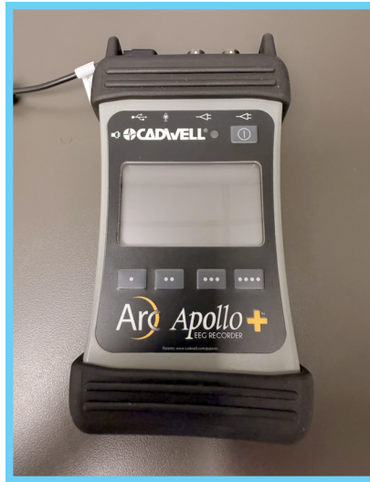
Portable EEG amplifier used to record and display brain activity signals.
