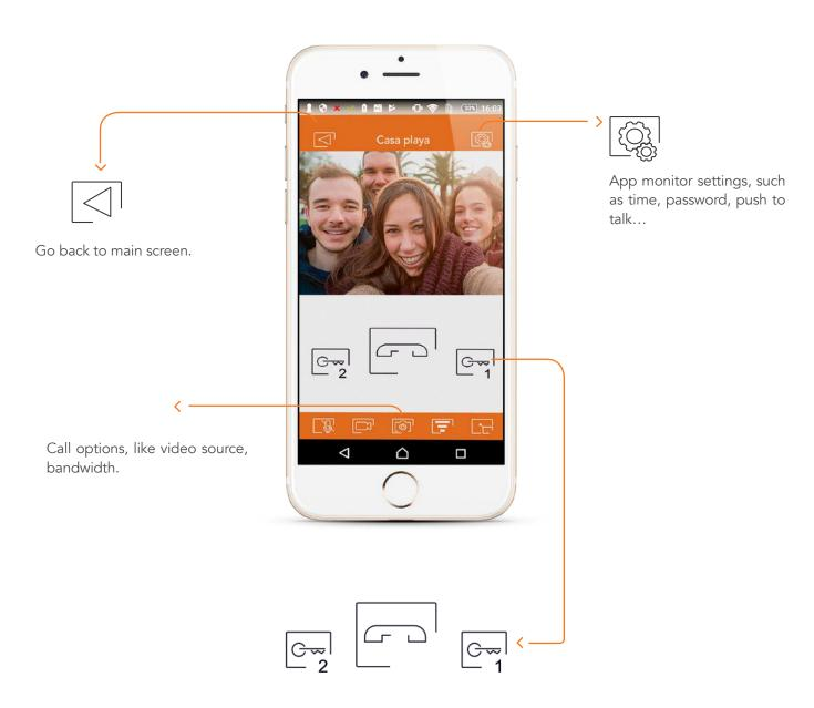
Communication menu, that allows to activate two doors and start or finish the communication.
