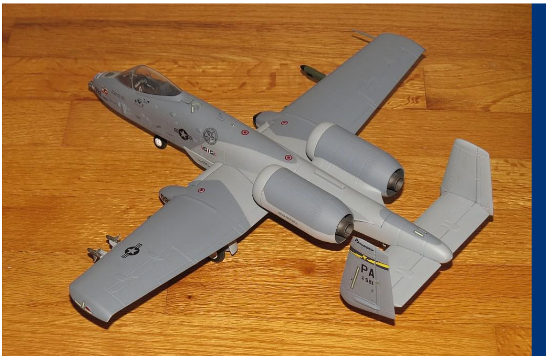
Franklin Mint's 1/48-scale Fairchild Republic A-10C Thunderbolt II die-cast model captures the unique look and features of the aircraft affectionately known as the "Warthog" well. The A-10s large General Electric TF-34-GE-100A turbofans are positioned above the fuselage to minimize the possibility of damage from debris when the aircraft is operating from unprepared runways. The twin tail configuration of the A-10 helps deflect the exhaust of the engines and reduce their heat signature
