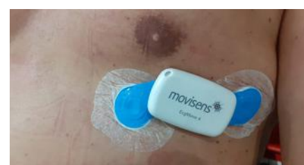
The movisens EcgMove 4 device used for data collection applied on a volunteer diver's chest.
