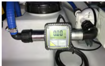
Meter FMT 3 with pulse output
