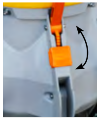
Spreading quantity adjustable with fixed stop
