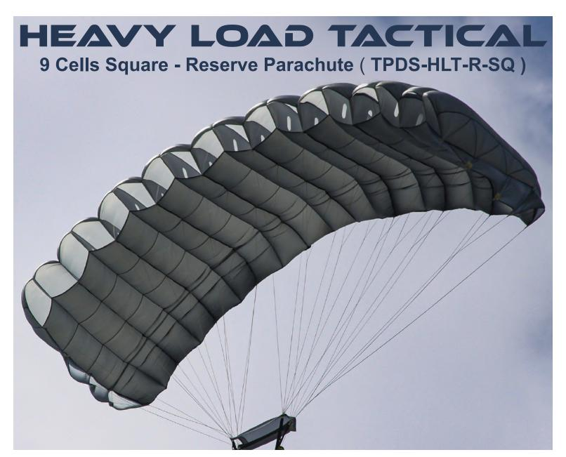
The TPDS-HLT-R-SQ is a nine-cell square ram-air reserve canopy purpose-built for tactical heavy load missions, ensuring reliable deployment and stable flight behavior during emergency scenarios. Sized between 300 and 460 square feet, it is matched to the main canopy's operational envelope, supporting both dual personnel and heavy equipment profiles without compromising performance.
