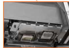
Staggered Dual Print Heads
