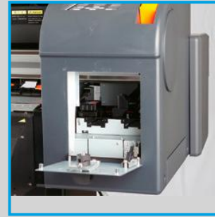
Maintenance access door
