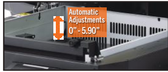
Automatic table height control from 0"-5.90.
