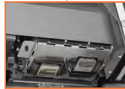
Staggered Dual Print Heads
