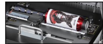
ROTARY UNIT Enables printing on cylindrical objects.
