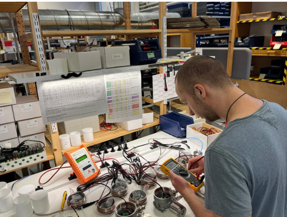
A technician checking sensor stability in newly manufactured gas detectors
