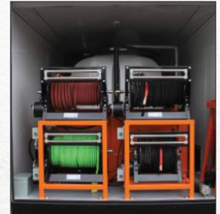
Wet Steam - Jetter & 2 x High Pressure Hose & Reels
