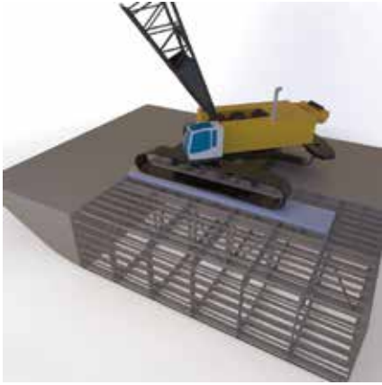
Renderings of a barge's inner structure – steel frames, ballast tanks for balance, and a strong support structure built to hold heavy cranes.
