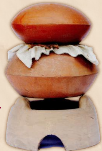
Patana Yantra ▶ was used for sublimation and distillation
