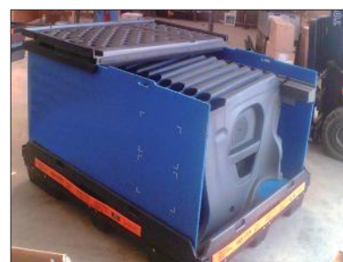
Pallets with Aircell collars and lids combined with a foam interior to keep automotive parts in place.
