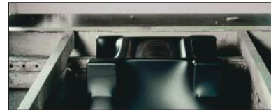
Then the mould rises and the air is sucked out of the machine.
