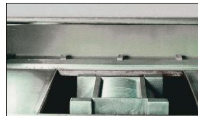
After the product has cooled, the mould goes back down and the plate is removed from the machine.
