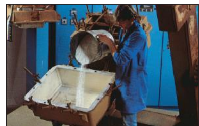
The mould is filled and then closed.
