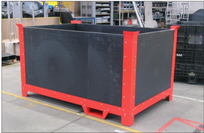
"Silent" collection bin for steel scraps made of a metal frame with plastic panels. Designed for Volkswagen.
