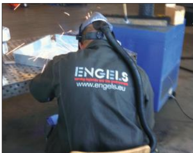
Welding of aluminium. Many of our products are made of aluminium because of its low weight and good corrosion resistance.
