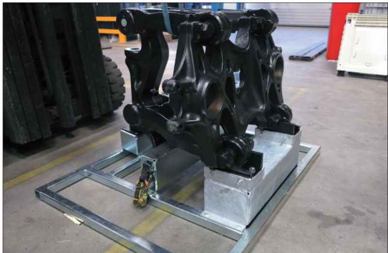
An all-steel product carrier for an agricultural vehicle component. The product carrier is adapted for use with a Smartbox.
