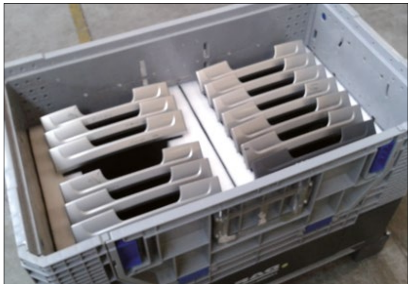
Corrugated plate inserts combined with foam for interior part truck cabin.
