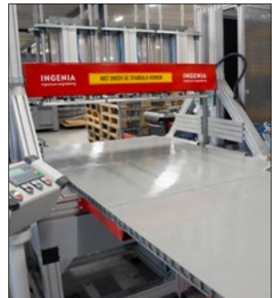
Mirror welding machine for welding plastic products up to 1200 x 1000 mm.
