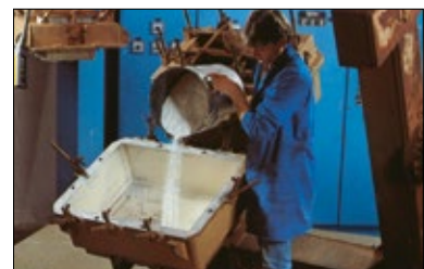
The mould is filled and then closed.
