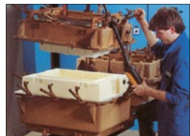
After cooling, the hollow product is removed from the mould.
