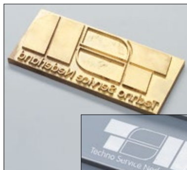
Customisation: printing by means of a cliché.
