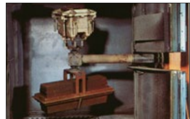
The arm rotates in the furnace, the moulds in turn rotate around the arm.
