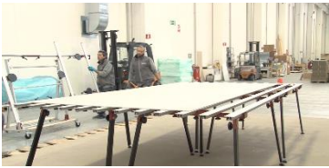
Workbench with aluminium profiles
