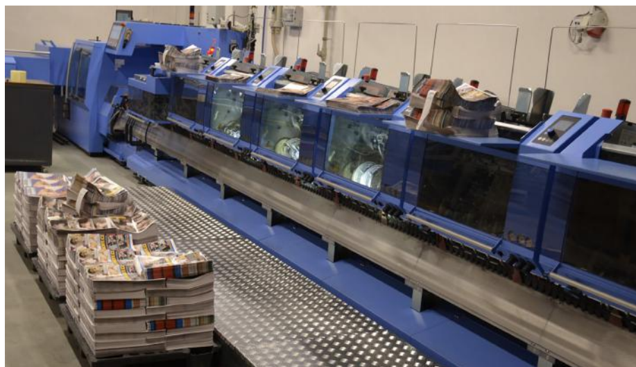
Triangl Print also relies on three Muller Martini saddle stitchers in its two plants – one Primera PRO (pictured) in Prague and two Primera machines in Milovice.
