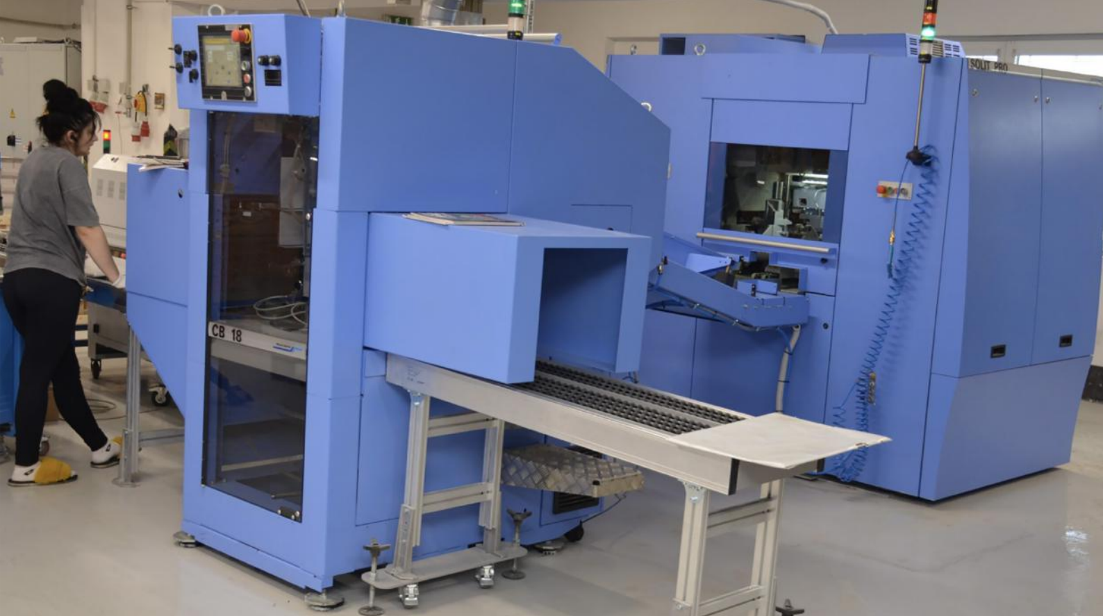
The Solit PRO three-knife trimmer ensures a clean cut, while the CB 18 ensures perfect product stacking.
