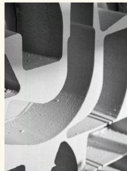
Carved cavity on the foam stock after CNC subtractive process
