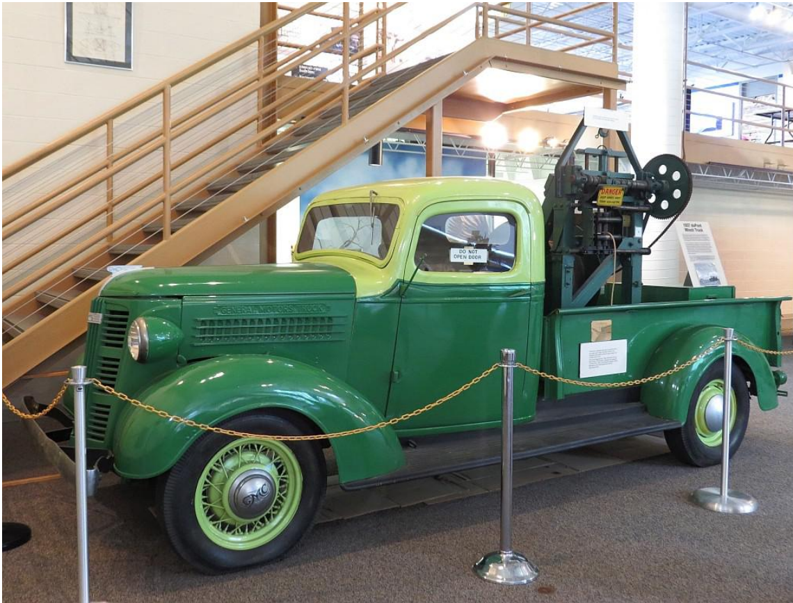
This 1937 GMC pickup truck was fitted with a winch designed by Stephen du Pont to launch gliders and sailplanes from the Harris Hill Gliderport. This winch truck was used to launch gliders and sailplanes at the gliderport during the first National Soaring Contests held in Elmira in the late 1930s.
