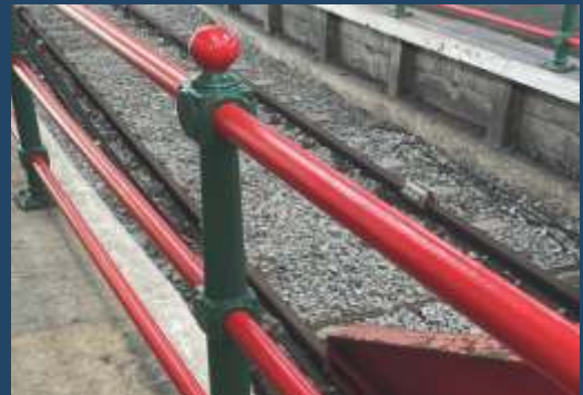
Mild steel substrate with aluminium rich epoxy primer containing zinc phosphate & 5% Intelli-ion® AX1 + topcoat
