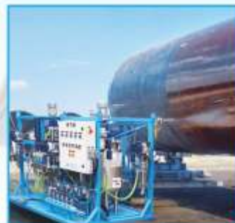
External Automatic Pipe Coating
