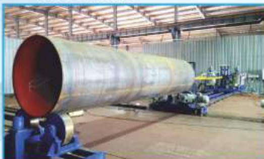
Internal Automatic Pipe Coating attachments and Boom Track Systems
