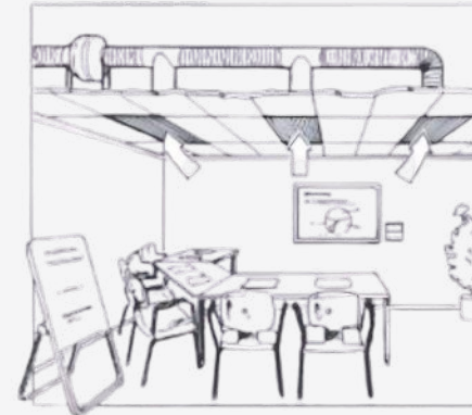
CONFERENCE ROOM EXHAUST VENTILATION
