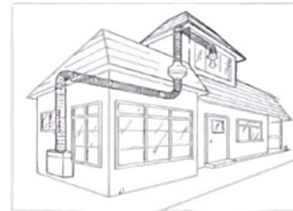
AIF FAN TRANSFERRING CONDITIONED AIR TO NEW ROOM ADDITION
