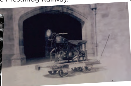
This run-about was built in the metalwork room with Mr McIvor - it was powered by a motorbike engine and was designed to run on rails when they were working on the Ffestiniog Railway
