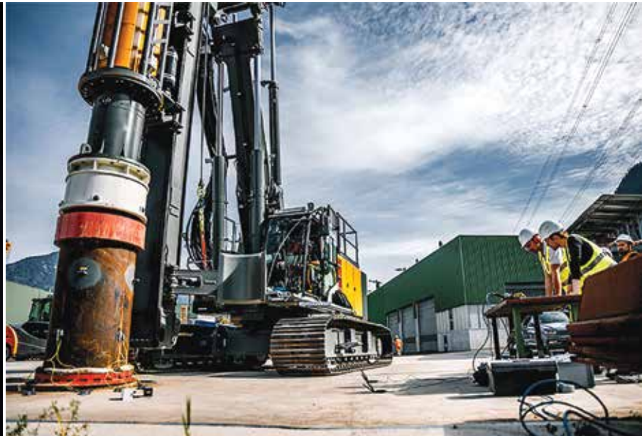
The combined piling and drilling rig LRH 200 offers flexible leader kinematics enabling very high radii and inclinations of up to 18 degrees in all directions.
