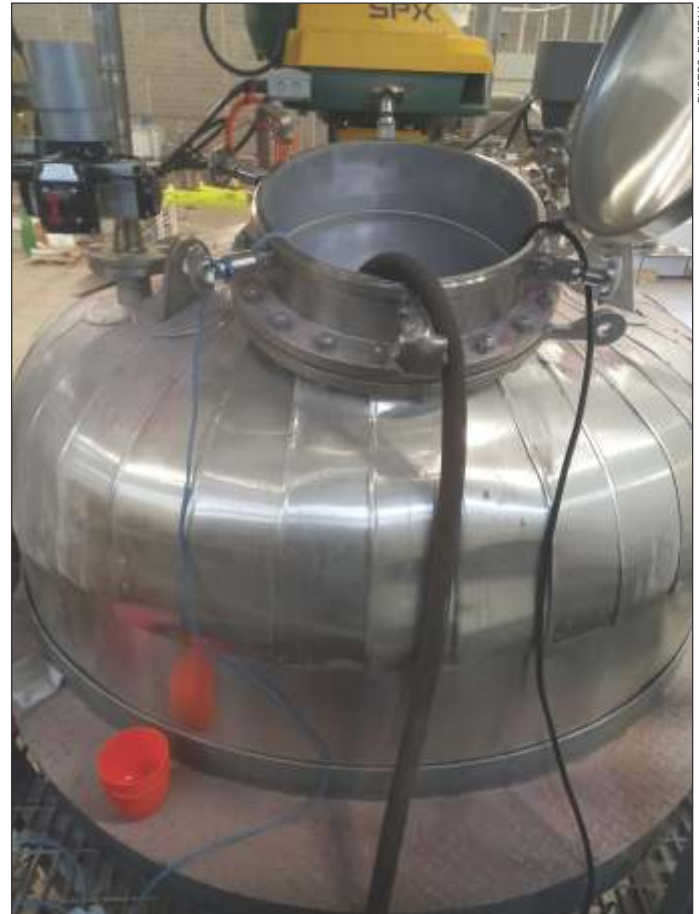
Figure 2: Tank used in process of creating biopolymer, chitosan.
