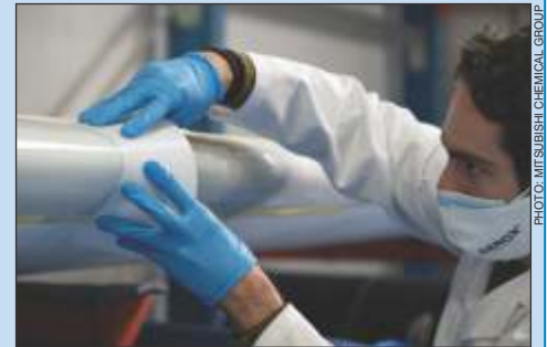
AEROX's AROLEP® 940 series coatings are used to protect the leading edges of wind turbine blades, for which the resistance against wind and rain erosion is necessary.
