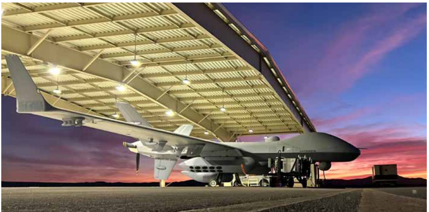
MQ-9B SeaGuardian equipped with a sonobuoy dispensing and monitoring system during testing in January 2026.
