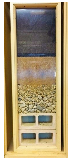
FILTERS 1-4 MEDIA&UNDERDRAIN SYSTEM
