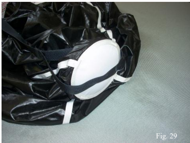
Go all the way up to the top of the Pilot Chute and pass the Pilot Chute through the loop of the bridle. (fig. 29)
