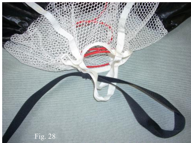
To attach the Pilot Chute, route the other end of the bridle through the two tapes of the Pilot Chute. (fig. 28)
