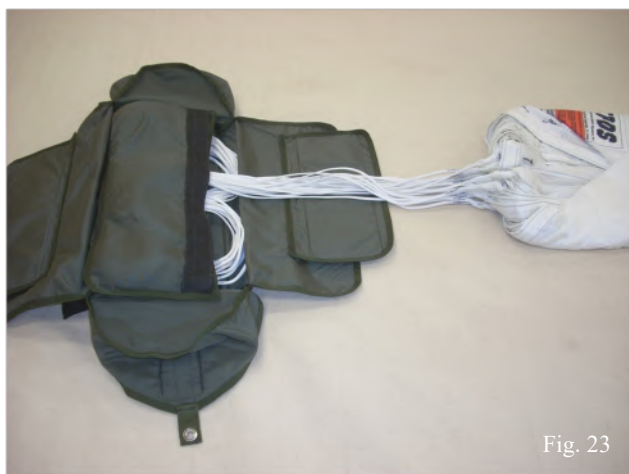
Leave approximately 12"-15" of line out of the pouch. (fig. 23)
