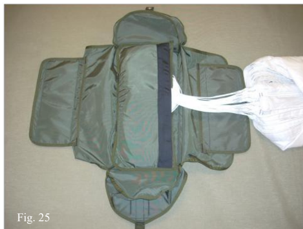
Mate the Velcro of the Pouch. (fig. 24)
