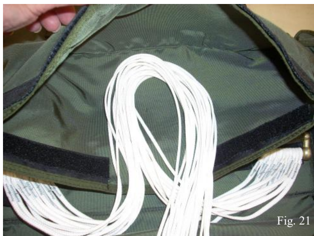
Place the lines into the pouch to the bottom of the pouch. (fig. 21)
