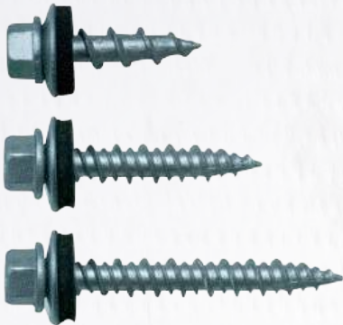
Hex Washer Head, AF 1/4", #8 Washer, Metal to Wood Screw, Type 17 Cutter
