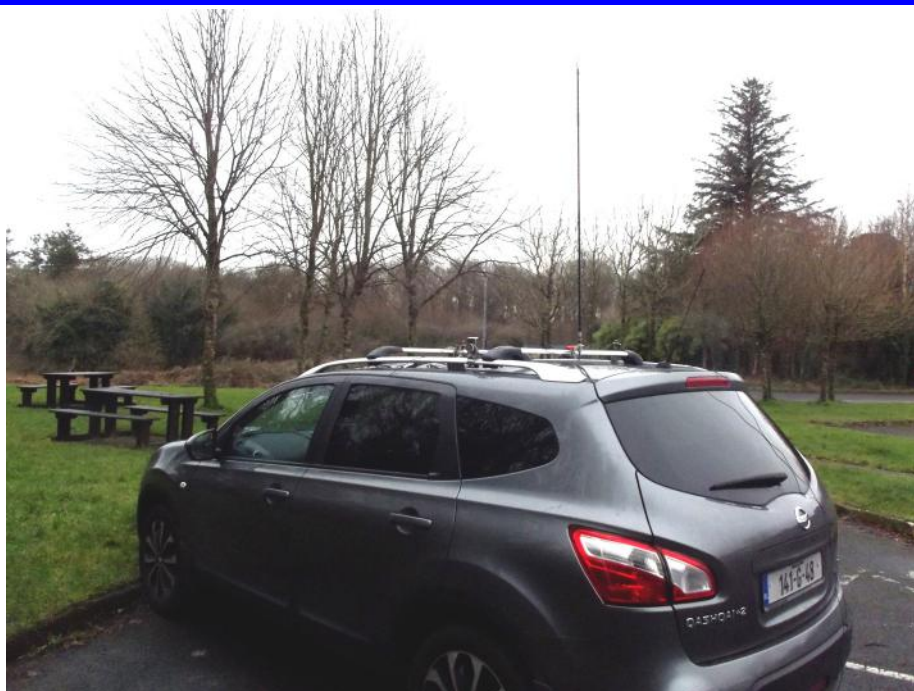
Using a Pro-Am Whip on 20 metres. Important to have a good earth so employed three radials clipped to base which made the antenna easier to tune
