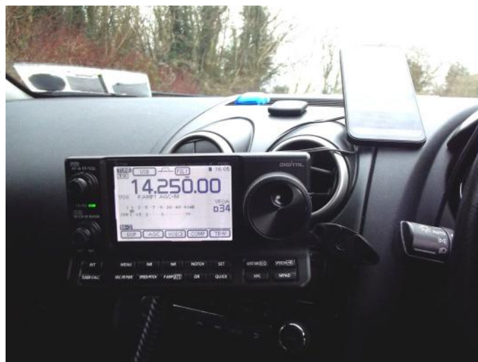
The ICOM IC-7100 is an excellent radio for POTA operation. The main body of the radio is mounted in the boot with the MAT Tuner. The tuner is not used with the Pro-Am Whip.
