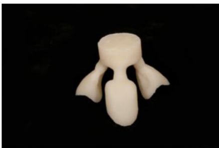
Divested units - see angulation of sprues
