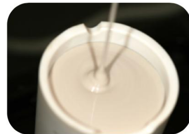
Fill up the ring up to upper line on the inside of the silicone ring
