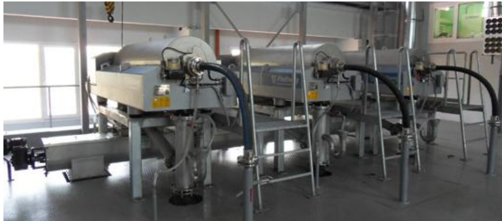
The Flottweg C Series decanter is a closed system, minimising odour and exposure to pathogens
