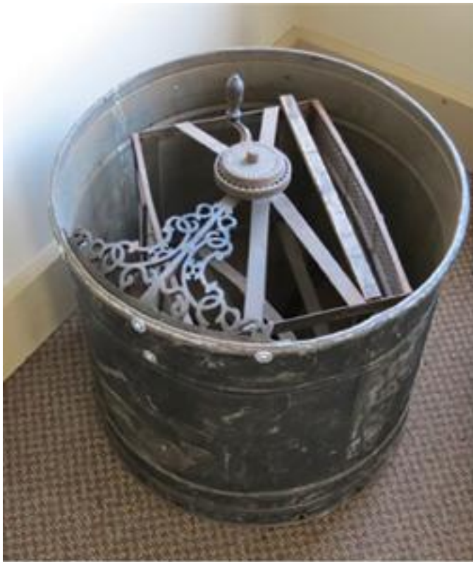
Novice Extractor - No. 2 for the American Frame or for any frame that is less than 12" long and 12 1/2" deep
