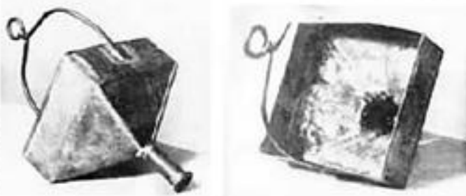
Device that Hruschka demonstrated the centrifugal force on uncapped honey comb.
