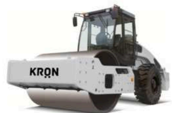
Road roller (soil) KRON SC12
