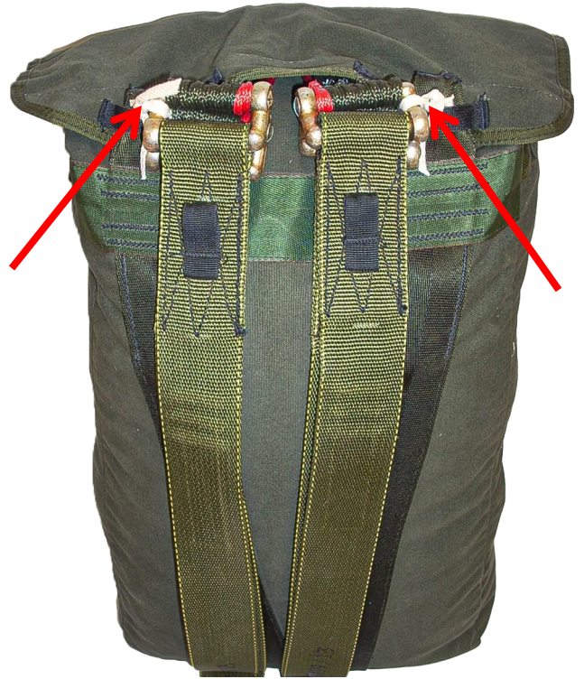
Riser to Deployment Bag 80 lbs. Break-tape
